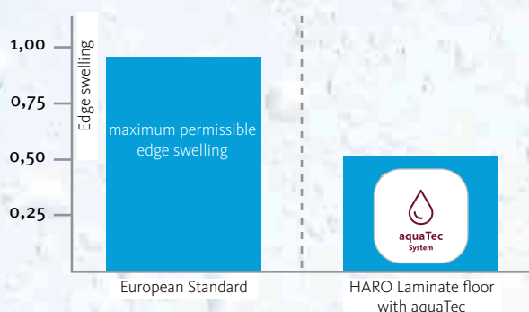
Laminate floor edge swelling with the effects of water
