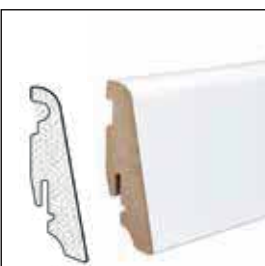
Stick-on skirtings, MDF core with laminate cover, 19x58 mm
