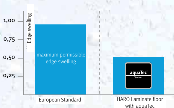
Laminate floor edge swelling with the effects of water
